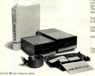
Introducing the Micropolis MacroFloppy™:1041 and :1042 disk drive subsystems. For the S-100/8080/Z-80 bus. Packing 100% more capacity into a 5%-inch floppy disk than anyone else. 143K bytes, to be exact. For as little
